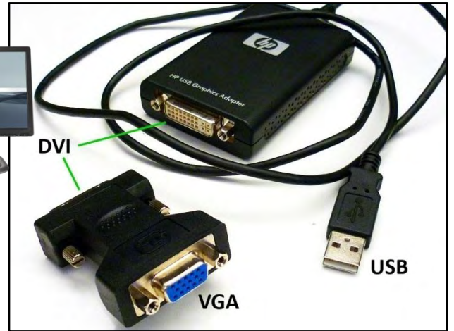
HP USB Graphics Adapter shown with USB cable and DVI to VGA adapter
